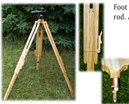
Foot modification - drill and tapped wood for 3/8-16 threaded rod. Added nut retains copper cap.
