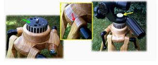
Added wooden spacer allows for more tripod head clearance. Manfrotto head adapter (green arrow) acts as additional spacer - 3/8 bolt extends thru all 3 pieces. Thin rubber washers (red arrow) between legs and tripod top plate to give the legs a lot more rigidity when tightened. Bubble level was epoxy glued in place.
