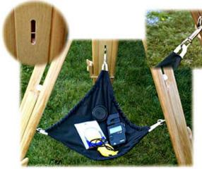
Routed small slits in legs provide access to metal pins inserted crosswise in the legs. Cloth shelf is attached by removable clamps (in order to reverse the legs). Shelf remains connected when tripod is folded.
